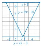
To graph y = |2x - 3|, graph y = 2x - 3, then reflect, in the *x*-axis, the part of the graph that is below the *x*-axis.
